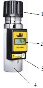
Figure 8. Wile-55 moisture meter: 1 – case cover; 2 – digital indicator; 3 – control panel; 4 – test sample container
