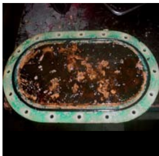
Figure 3. Microbial pollution of fuel tank
